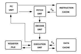
Figure 5. PDLX Microprocessor Block Diagram : top level view.
